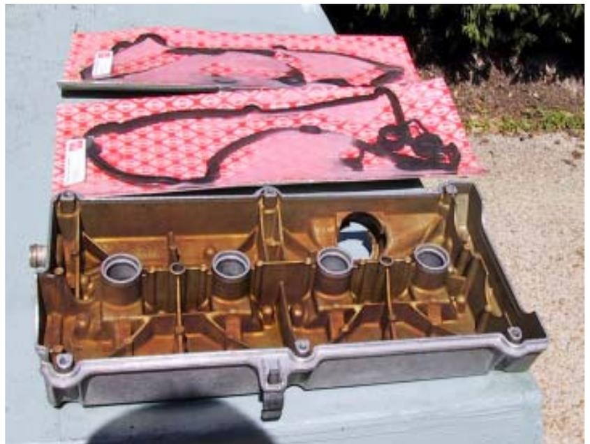
*Backside of Audi A8 valve cover and replacement gaskets. When replacing the gasket, ensure the valve cover and cylinder head are completely cleaned before installation of new gaskets.*
