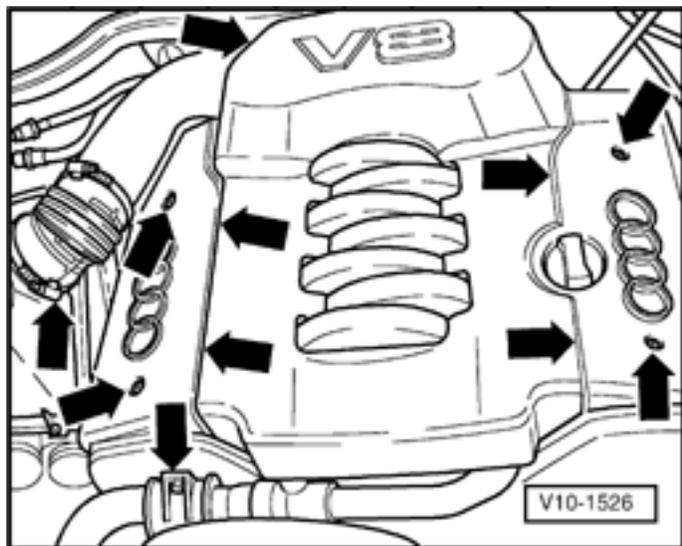
*The first step is to remove the engine plastic. Pull the side pieces first, then the center piece. Loosen intake hose clamps; remove hose and set aside. Stuff a paper towel into both the throttle body on engine and mass air sensor on air cleaner housing.*
