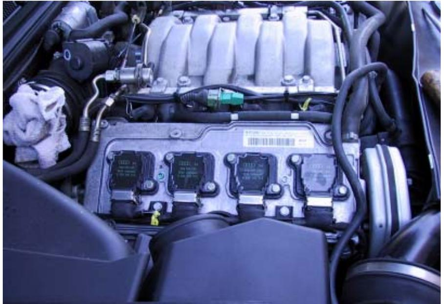
*Right hand valve cover. Note each coil is bolted in place, fuel lines are above and on the left, engine throttle body is stuffed with rag, and valve cover breather hose is on the front end of the valve cover.*
